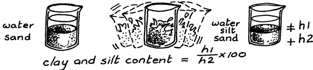
**1** - Take a **sand sample** as described below and fill one half of a **glass jar** with the **sand**. Add **water** to 50% above the sand level and **shake the jar** strongly for 30 seconds.
