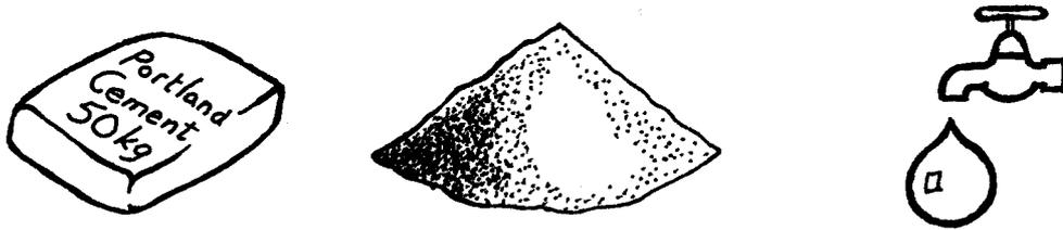
***Tile mortar is made by mixing cement, sand and water together.***
