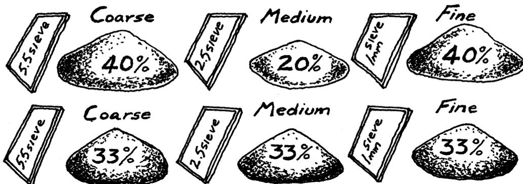
Try different **sand mixes** and make **sample tiles** to check the **workability** of the mortar - break these tiles after 28 days to measure their strengths and see which sand mixes produce the strongest tiles.
